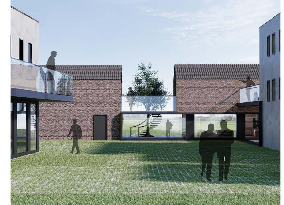
In Farmer and Manor house, by eliminating some walls and replacing them with proper columns, the design tries to form new modern spaces. However, by keeping some windows and bearing walls we wanted to respect the current definition of these buildings
